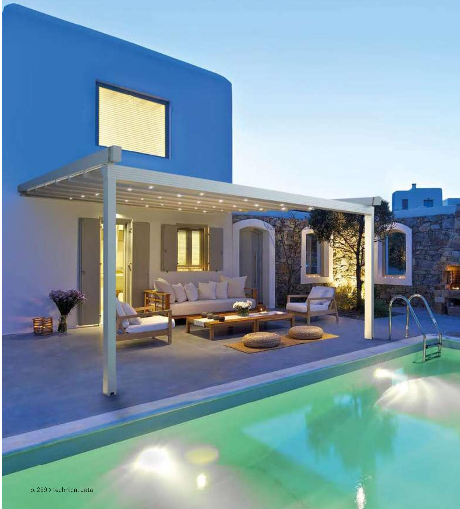
**Pergola in powder coated aluminum with strong, refined lines, with a structure with painted aluminum gutter. Available in wall mount, ceiling or self-bearing version (Pavilion model). The structure is equipped with a diamond frame, a PVC sheet cloth and front gutter with water drainage integrated in the posts. For a proper discharge of water, it must be installed with a minimum slope between 8% and 19% depending on the projection.**
